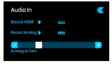
It is not possible to vary the gain if the signal input is from the HDMI connection because this is digital and is embedded in the signal. You can usually adjust this from the camera, see your cameras manual for operational details.
