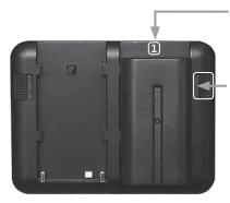
Battery number 1 Gently slide down into battery slot/s and lock into position.
